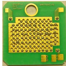
Fig. 2 Dispensed solder paste
