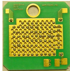
Fig. 2 Dispensed solder paste
