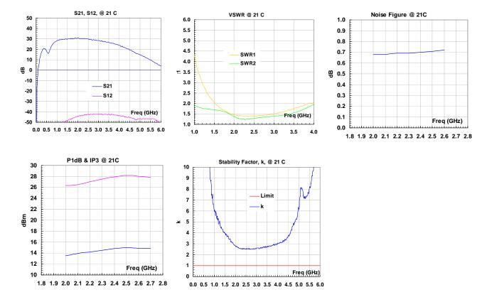
\*The measured noise figure includes the WP-5 test fixture and motherboard.
